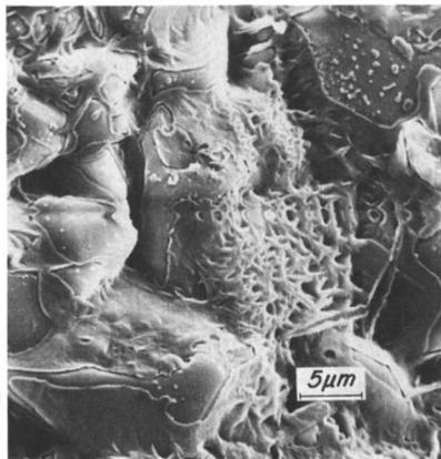
*Figure 13. Exterior surface of a coating with intergranular pores and poor mosaic texture*
