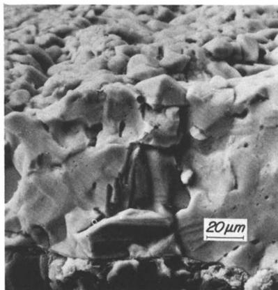
*Figure 18. Cross section and exterior (top) surface of massive sulfur texture in high-temperature coating allowed to cool slowly*
