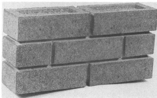
*Figure 2. Sulfur-bonded prefabricated brick panel*
