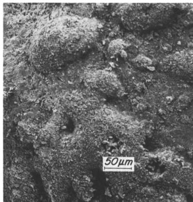
*Figure 12. Coated urea granule showing coalescence of sulfur droplets on the exterior surface*
